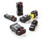
AMPSEAL 16 hybrid lever is a sealed connector system that features a lever slide mechanism for mating and a slide-in mounting clip. The mix of 24 x size 16 and 4 x size 12 terminals creates design flexibility for use in various vehicle applications.
