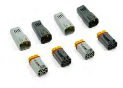
Using the proven MCON 1.2 SWS terminal with a 17 A-current carrying capacity, SUPERSEAL pro 2-, 3-, and 4-position sealed connectors provide a vibration resistance that complies with USCAR V2. With pre-assembled and color-coded TPA options, SUPERSEAL pro's integrated front seal housing design improves terminal retention and allows easy assembly.
