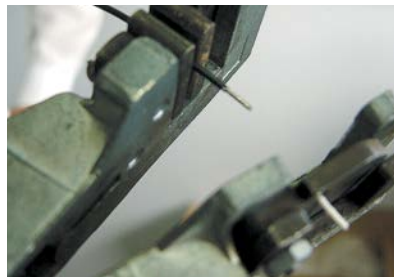
Wire stripping with a recommended tool will allow the insulation to be removed accurately without damaging the wires.
